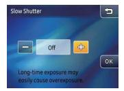
To set the exposure time: Touch the or button to adjust the exposure time. Press and hold the button for 2 seconds to automatically increases / decreases the exposure time to the limit between 2 to 30 seconds.
